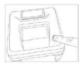
e) Removing jammed paper: Open the cover to remove jammed paper. Check if the printer head is not contaminated, if yes, clean it with cotton swab moistened with an alcohol solvent (ethanol or IPA). Wait until alcohol will completely vaporize and then close the cover.
